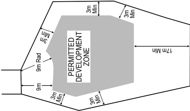
Fig. 3 Plot in "Hammerhead" of a Cul-de-Sac
